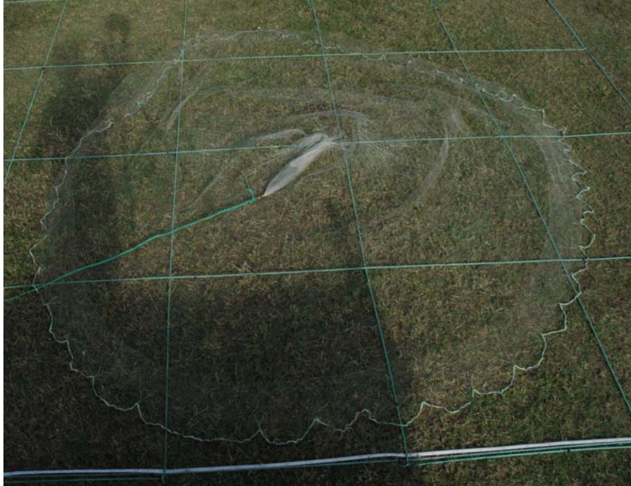
Figure 9: Example of cast net used for nekton surveys
